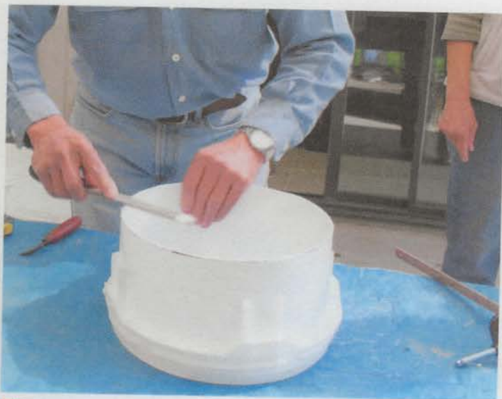
5 File or sand off the rough edges.
