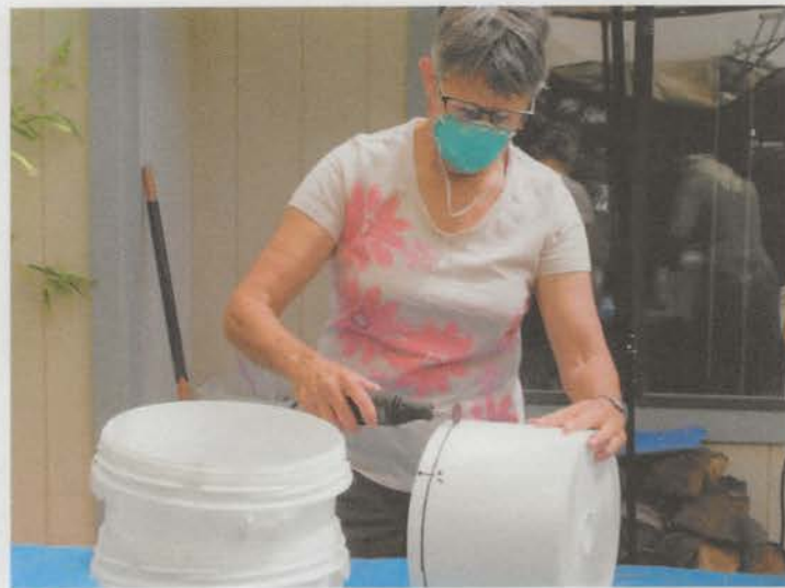
13 Cut the ring band using a Dremel saw (alternative to hacksaw).
